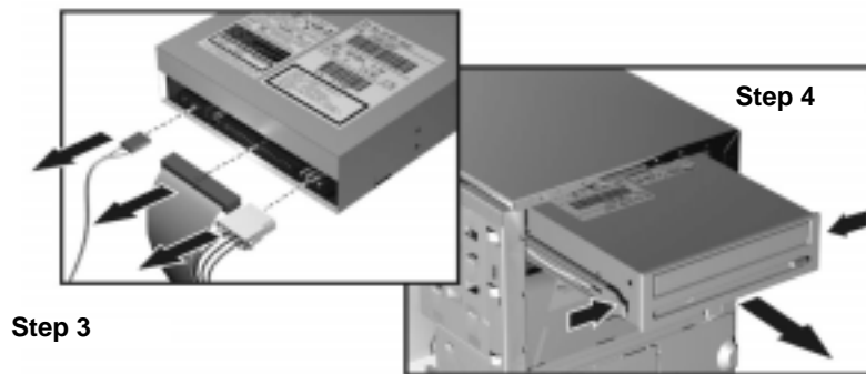
Figure 10-20 Removing the Old Drive
